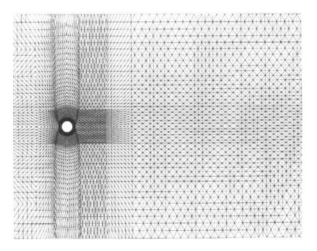
Figure 2. Finite element mesh for blockage ratio 0.05
