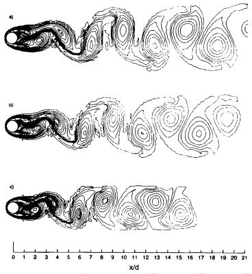
Figure 15. Equivorticity lines for unsteady flow: (a) d/h = 0.05; (b) d/h = 0.15; (c) d/h = 0.25
