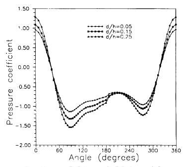
Figure 16. Pressure distribution around cylinder for unsteady flow
