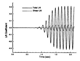
Figure 12. Time-dependent lift coefficient on cylinder; d/h = 0.25
