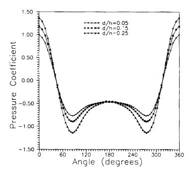
Figure 6. Pressure distribution around cylinder for three blockage ratios
