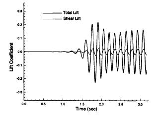
Figure 11. Time-dependent lift coefficient on cylinder; d/h = 0.05
