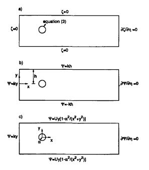
Figure 1. Boundary conditions: (a) vorticity; (b) streamfunction; (c) streamfunction from irrotational solution at outer boundaries.
