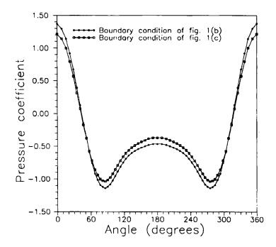
Figure 8. Effect of boundary condition on pressure distribution around cylinder; d/h = 0.25
