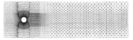
Figure 3. Finite element mesh for blockage ratio 0.15
