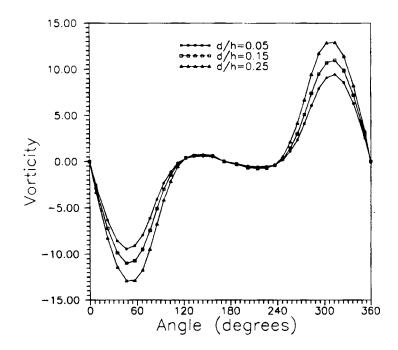
Figure 7. Vorticity distribution around cylinder for three blockage ratios
