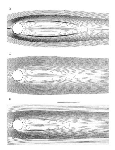
Figure 5. Streamlines for steady flow: (a) d/h = 0.05; (b) d/h = 0.15; (c) d/h = 0.25
